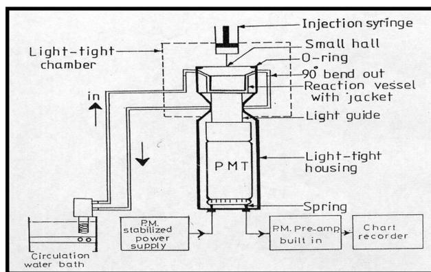
**Figure 1** - Schematic diagram of the photon counting system.
