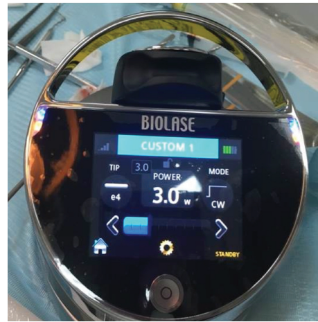
Figure 2 - Biolase ePic 10 Diode laser 940nm, showing the applied Laser parameters
